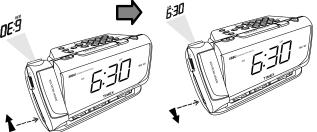
4. If the image is fuzzy or out of focus, slowly rotate the FOCUS adjustment ring clockwise or counter-clockwise until you achieve the sharpest focus.
